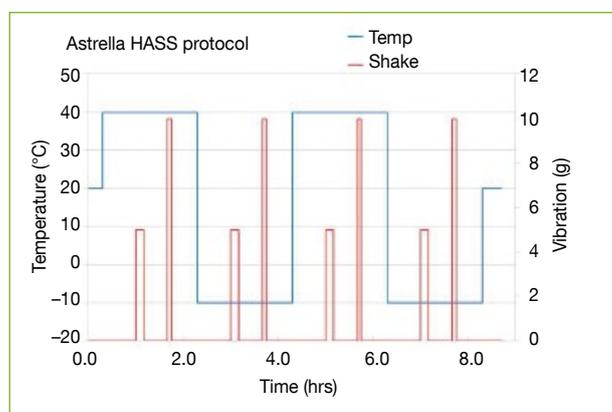
Fig. 4 The HASS test protocol current used for every single unit of a new type of short pulse (< 35 fs) ultrafast amplifier – Coherent Astrella.
