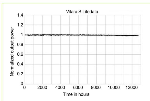
Fig. 3 Vitara-S life test run at constant pump power.
