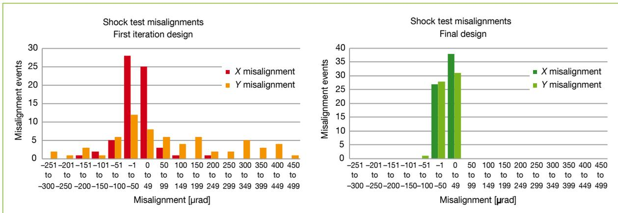
Fig. 2 Comparison of an earlier version of optical mounts with the final version used in femtosecond lasers. The final version is much more compliant with externally induced vibration and temperature change cycles.
