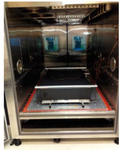
Fig. 1 The laser industry’s first ever HALT / HASS chamber enables testing of even large footprint products such as this Astrella one-box femtosecond amplifier system.
