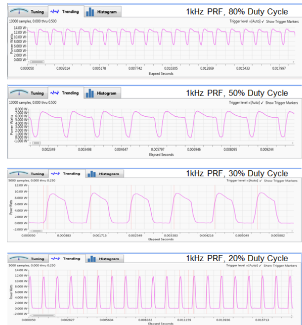
Figure 4 Pulse Shape Visualization Obtained with a PowerMax-Pro Sensor and LabMax-Pro Electronics and Software
